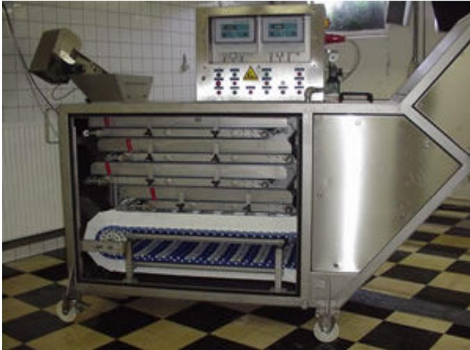
Due to years of research and the construction of several machines, the user-friendliness of the AED-10™ is optimal. For example, it is easy to clean the machine by removing its cover panels, giving access to parts inside the machine and making it possible to properly hose down every area of it.
