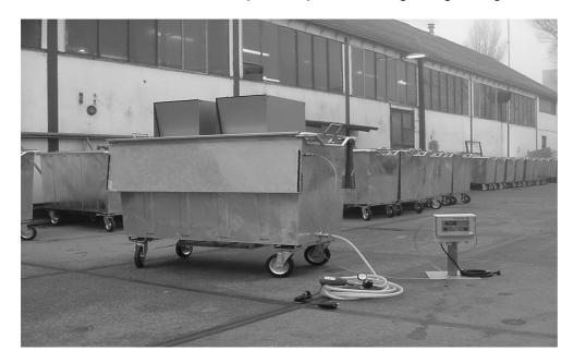
System : non-stop by means of 7 drums and 4 lids + analyser Capacity : 5000 – 7500 chickens or 300 – 500 turkeys per hour
